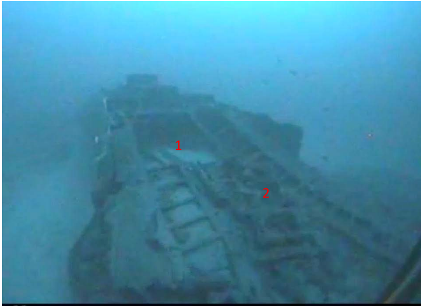
Figure 86: View aft hatch looking forward showing hatchway (1) and mast step (2) (Image: CSIRO 2023 - )
