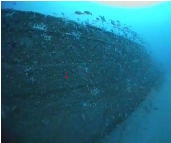
Figure 83: Main sheerstrake hull plating (1) on starboard side below the bridge (Image: CSIRO 2023 - Lapped Hull Plating Side cam)
