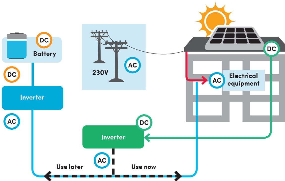
**Figure 4: An AC-coupled system with two separate inverters: one for the battery and one for the solar PV.**
