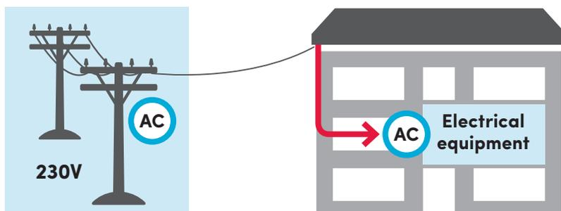
**Figure 1: Electricity is generally supplied to businesses in New South Wales as alternating current (AC) at 230 volts single-phase or 400 volts three-phase.**
