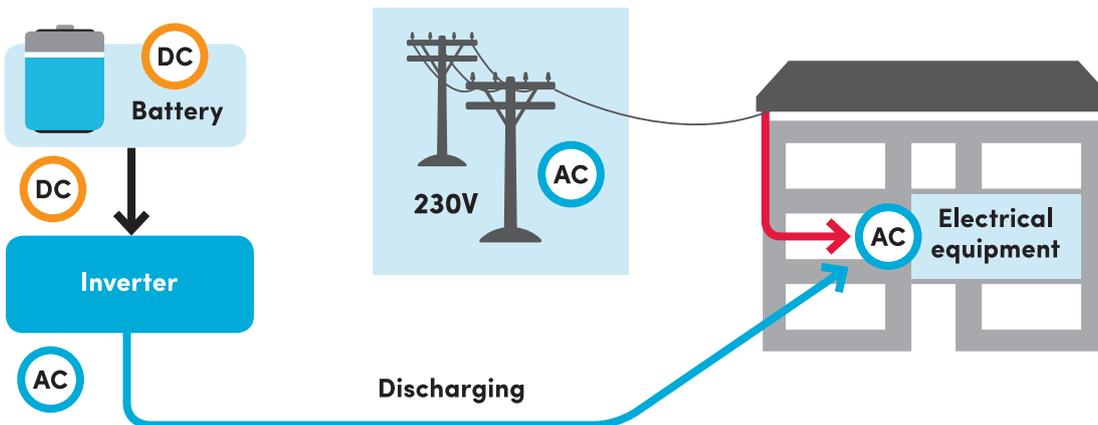
Figure 3: A battery system is designed to cycle between storing energy (charging) when the cost to do so is low and using the energy (discharging) when the benefit is high, for example, when the price of electricity is relatively high.
