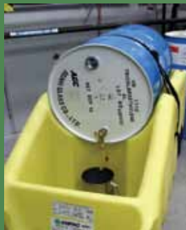
Mobile drum containment unit for spill control (DECCW)
