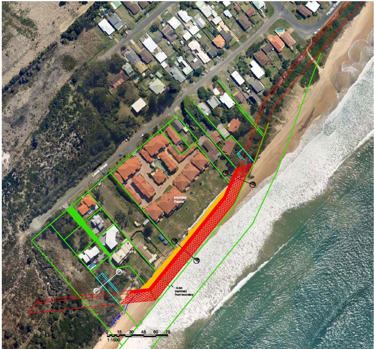
Figure 2 – Proposed return wall extension [extract from ICM drawing OB-EPW-005]
