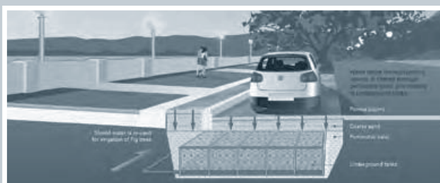
Rose Bay stormwater treatment and storage cells
