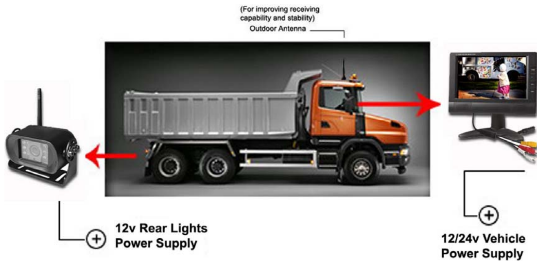
Figure 6.4: Example of a proximity detector combined with an in cabin camera display [Animedia Corporation, 2008]
