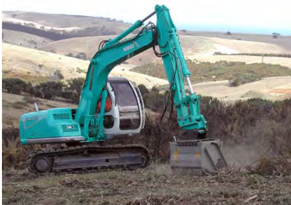
Groomers can be used on weeds such as gorse and brooms
