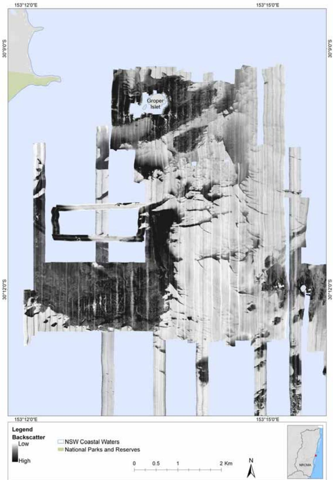
**Figure 28. Acoustic backscatter of the seabed adjacent to and south of South West Solitary (Groper) Island, including Sidney Shoals.**
