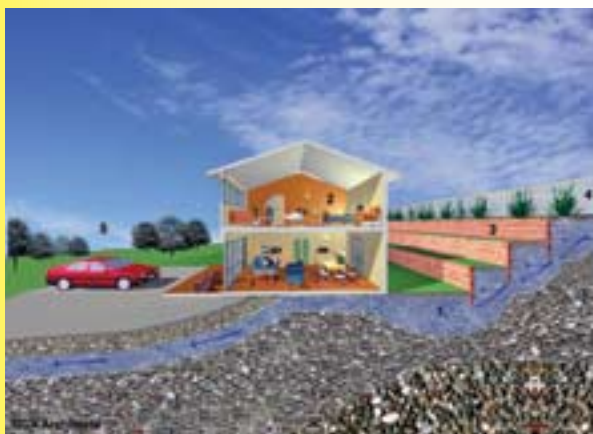
Water flow obstructed by urban development Diagram: DIPNR- Greener Subdivision project
