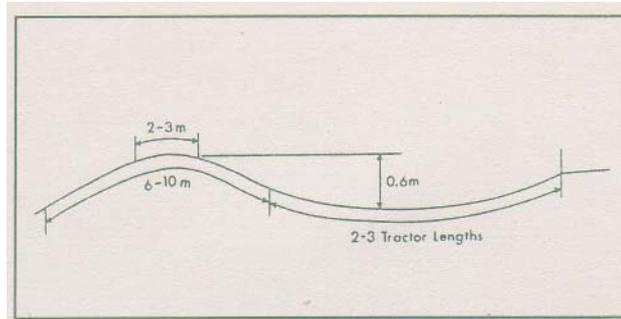
Figure 2: Dimensions of cross banks.
