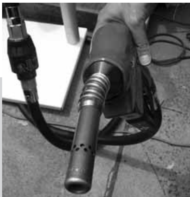
The holes in this nozzle recover vapour emissions before they reach the atmosphere.
