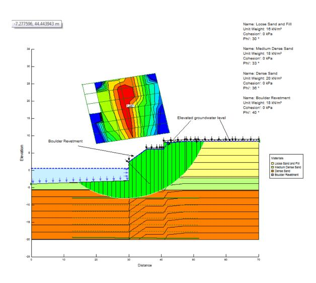
THEORETICAL SLIP CIRCLE – GLOBAL FAILURE PILE TOE AT RL – 8m WITH ELEVATED GROUNDWATER LEVEL
