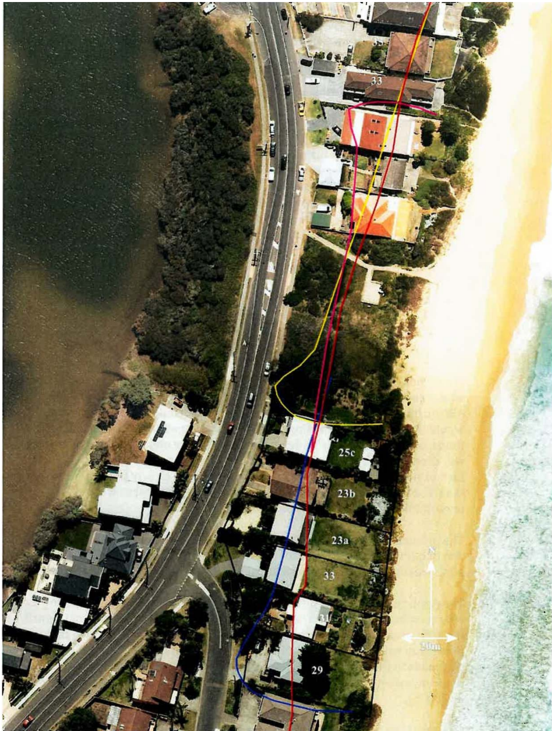
Figure 1: Indicative end effects related to existing and proposed protection works based on Carley et al (2013), with red line being the existing 100 year ARI storm extent of erosion, blue line being the existing end effect from the Manyana revetment, magenta line being the existing end effect from the 33 and 35 Ocean View Drive revetment, and yellow line being the end effect from the proposed revetment (2014 aerial photograph)
