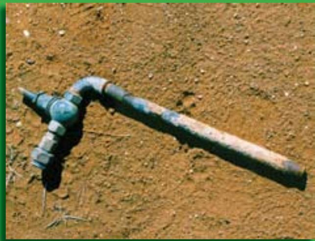
**Fig. 17** Premature corrosion and breakdown of a galvanized pipe due to high soil salinity. Photo: A. Collings
