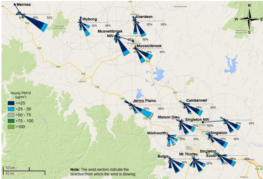
Figure 3 Hourly PM10 pollution rose map for the Upper Hunter region for summer 2022-23
