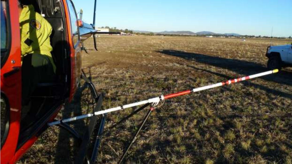
**Fig. 6** Sighting boom mounted on the left-hand side of the Eurocopter AS350 Écureuil helicopter. The perpendicular distance classes used in the surveys (0-20 m, 20-40 m, 40-70 m, 70-100 m and 100-150 m) are indicated by the black bands on the boom.
