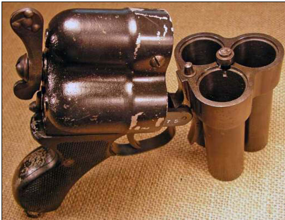
Figure 37: Triple Barrelled 28mm Type 90 Japanese Signal pistol Type 3 (Image: Courtesy Teri Byrant, http://members.shaw.ca/ursacki/fgtype90triple3vpix.htm ).
