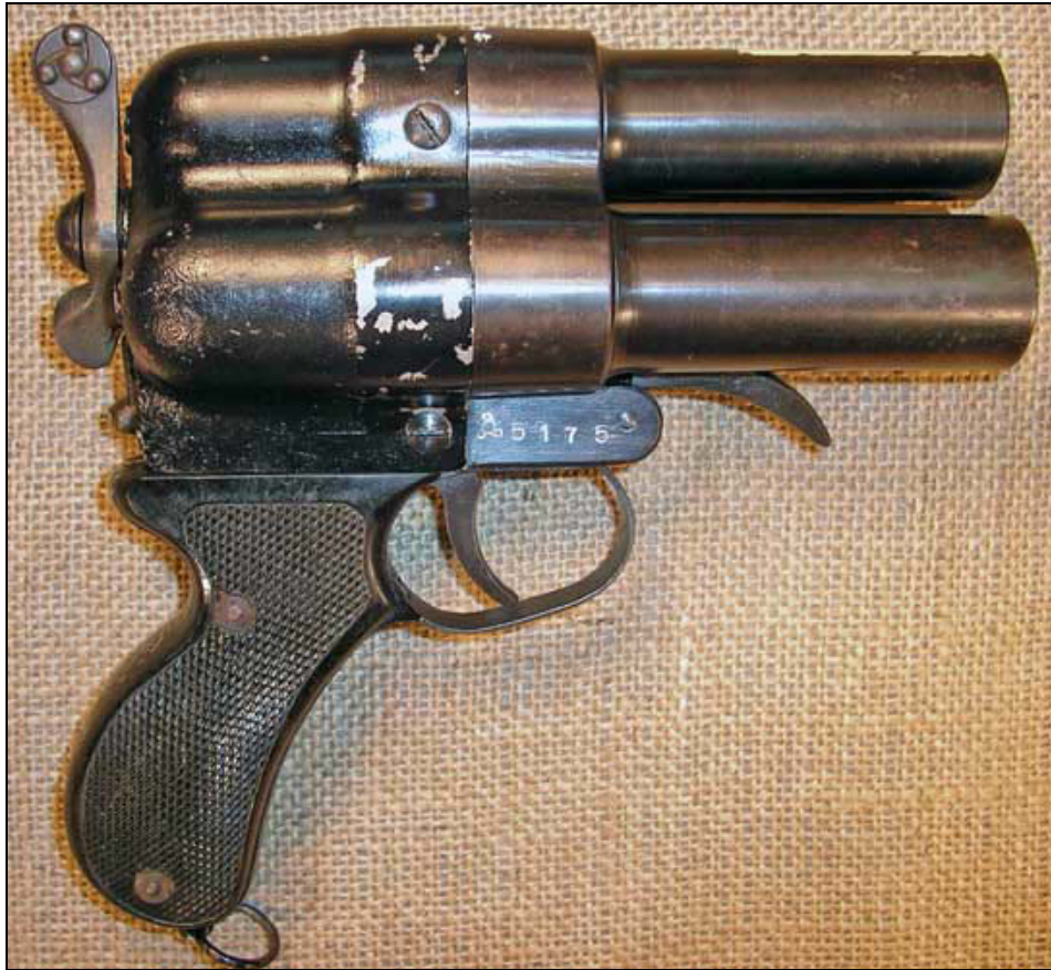
Figure 36: Triple Barrelled 28mm Type 90 Japanese Signal pistol Type 3 (Image: Courtesy Teri Byrant, http://members.shaw.ca/ursacki/fgtype90triple3vpix.htm ).
