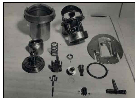
Figure 47: Dismantled inertia pistol mechanism from M24 torpedo at Garden Island (Image: from NAA #668555, Plate 34).
