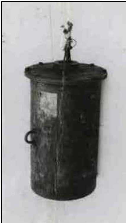
Figure 30: Side view of Japanese demolition charge, showing cover plate, safety fuse and collar (Image: After NAA# 400146).
