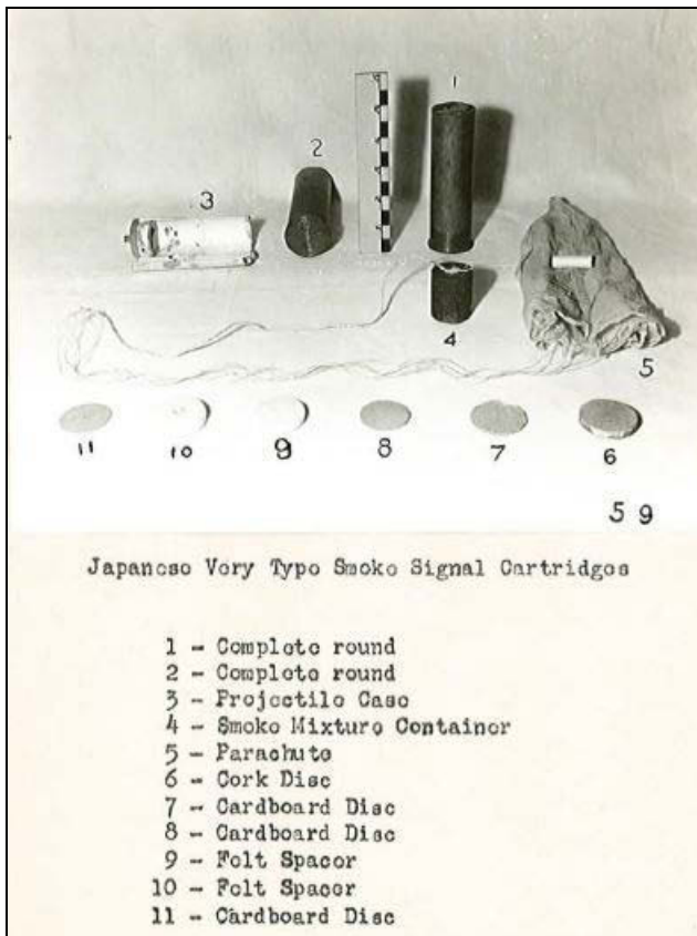
Figure 41: Physical composition of Japanese Very Smoke Signal Cartridge (Image: from Very Round Pistol Report - Hollandia AWM #54 179/1/25).
