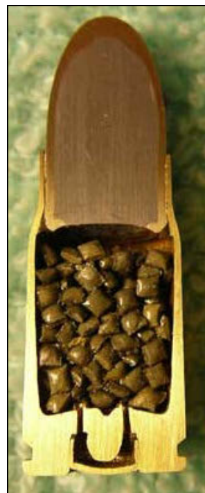
Figure 44: Cutaway section of a Japanese Nambu 8mm round (Image: After Bryant 2005).
