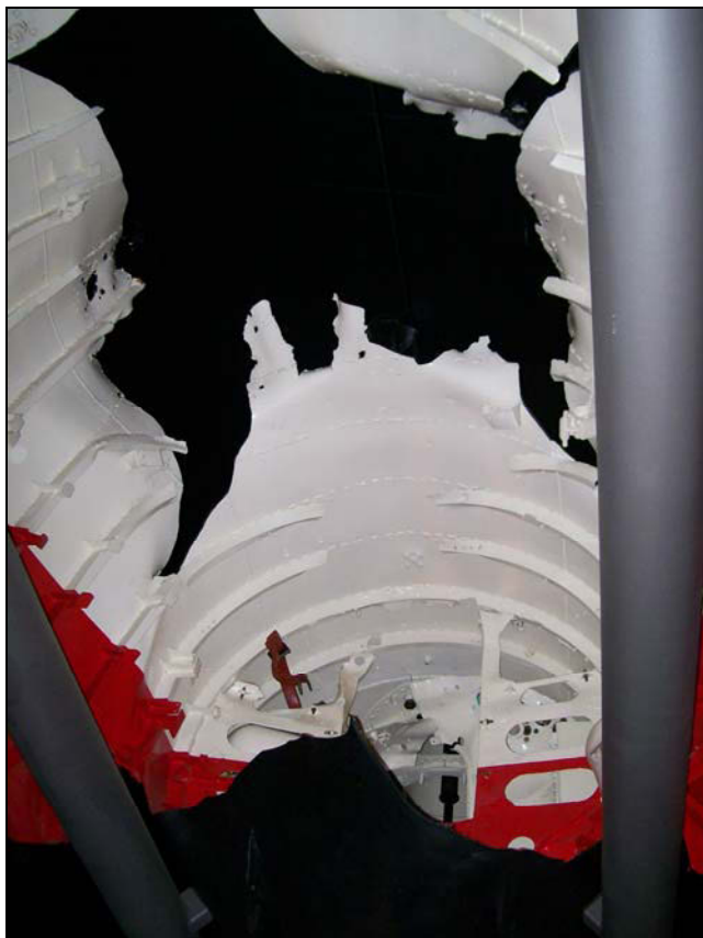
Figure 17: Inside Ha-14 aft battery room facing aft control room compartment bulkhead. Note the dark section of hull bent upward and inwards at the bottom of the image. On display at AWM, Canberra (Image: Tim Smith).
