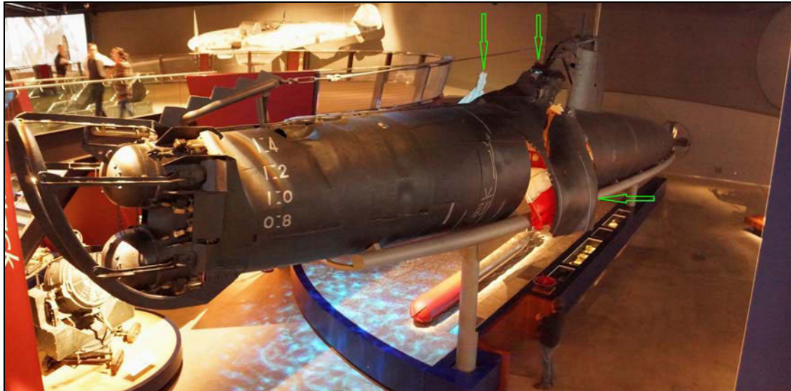
Figure 25: Bow section of Ha 21 and attached hull of Ha-14 hull looking aft. Note the evidence of upward explosion near conning tower (green vertical arrows) between frames 4-6 forward of the net-cutter. The athwart explosion is evidenced by a bulging/ bubbling with a distinct vertical line of the outer hull plates, which corresponds to frame 4 on the interior of the hull –see horizontal arrow. (Image: After Photomosaic by B. Duncan, Heritage Division).
