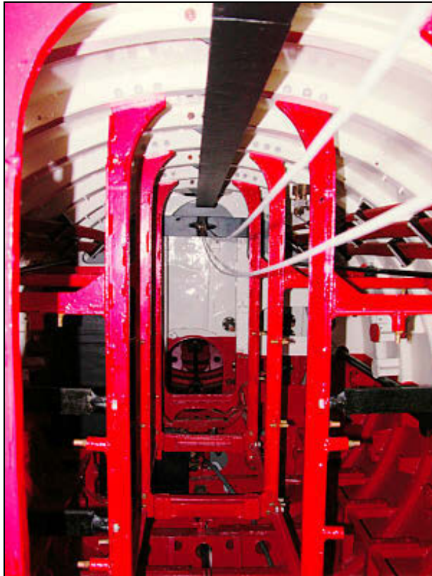
Figure 18: Aft battery room inside remains of Ha-21 (Australian War Memorial, Canberra. The aft scuttling charge is considered to have been placed within the floor passageway, possibly close to the control room bulkhead. The remains of the battery bank shelves are located either side of the companionway (Photo: Tim Smith).
