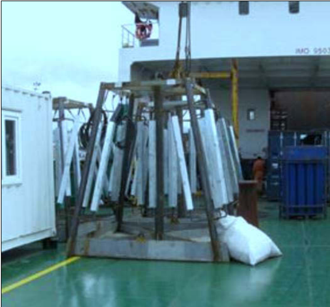
Figure 56: Anode Pod deployed on AE2 submarine wreck, Turkey (Image: After MacLeod 2015, Project Silent ANZAAC).
