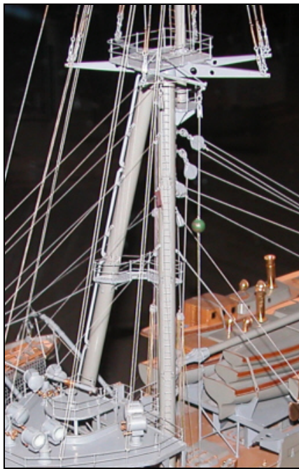
Figure 22: AWM model of HMAS Australia showing aft control tower top (platform) and ladder (Photo: Tim Smith 2007)
