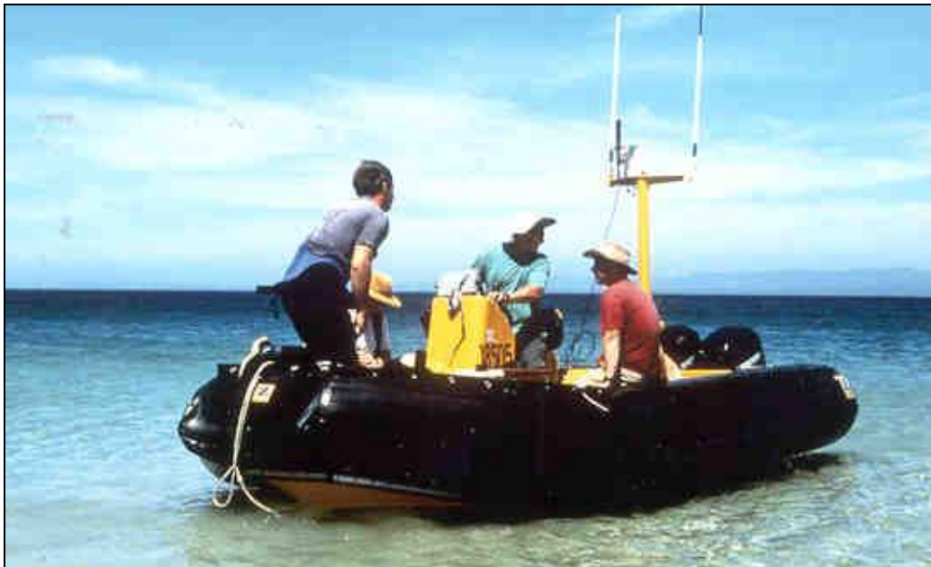
Figure 6: Manly Hydraulics Laboratory inflatable from which the Australian Defence Industries' Ferex magnetometer was deployed in locating the remains of the 'Hive' shipwreck.
