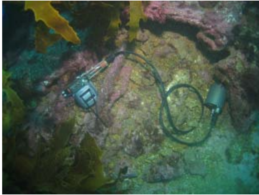
Figure 1. The fluorometer deployed at 24 m on the red alga Delisea pulchra . Note deployment is on part of the structure of the Duckenfield. The measuring tube is on the left connected by cable to the logger housing on the right. (Photo: Sterling Smith 2005)
