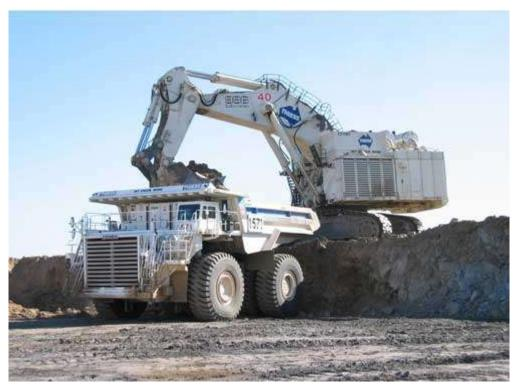
Figure 6 Large excavator loading haul truck
