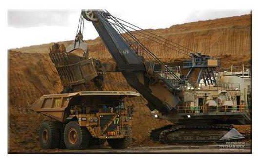
Figure 7 Hydraulic shovel loading haul truck
