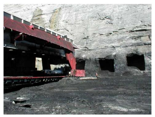
Figure 9 Highwall mining using an auger miner
