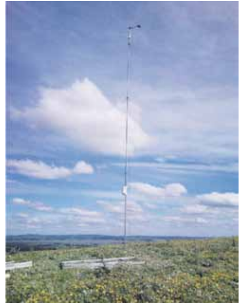
9m wind monitoring mast with Davis equipment
