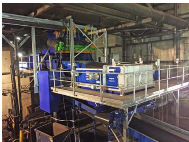
New machinery at the Global Renewables Eastern Creek facility extracts and cleans metals from mixed household waste, creating a high-value product for recycling and re-use
