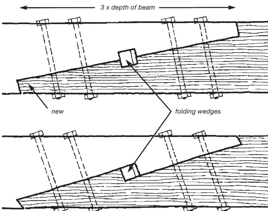
The timber species and moisture content of the new timber need to be carefully matched with the old to avoid differential movement. For clear-finished joinery, the colour and grain direction of the repair also need to be matched, and the new piece fitted to the old with a hairline joint.
