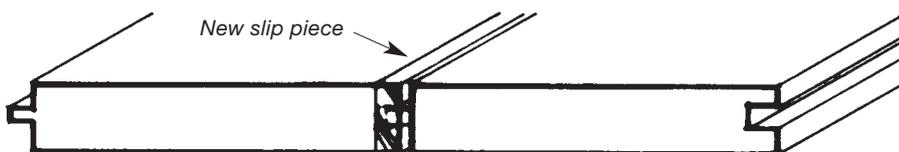
**Possible repair to the face of a board**
