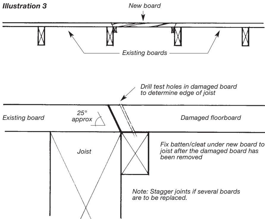
(c) Insert a strip (sometimes called a 'slip') of timber in the gap created. The strip should be of the same timber and section as the existing, and be fully seasoned. The strip will need to span the joists below. Note that smaller areas of repair which cannot span between joists can be done as dovetail and tapered splices (shown in illustration 3). This technique is also described in Information Sheet 5.3. *Patching Old Floorboards.*
