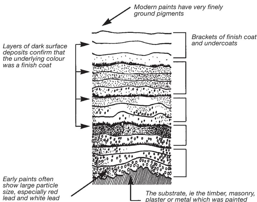
A magnified cross-section of a sample of paint built up over many years shows distinct patterns. The surface or finish coats are identified by the accumulation of dirt deposits which survived the painter's preparations, even on vertical surfaces.
