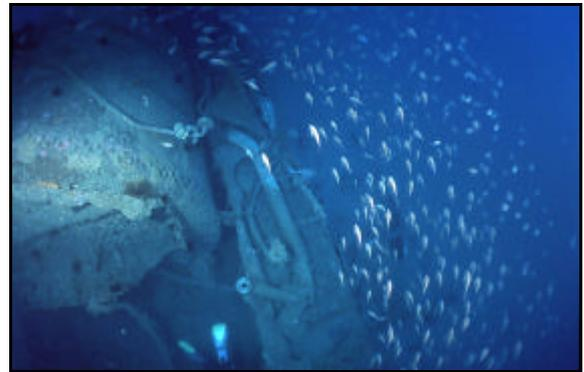
View of port side of hull, showing boiler (to left) and ship's funnel lying on sand in centre. Copyright Mark Spencer.
