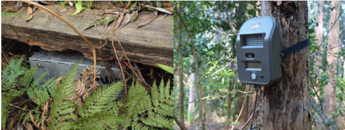
Targeted survey techniques included setting Elliott A traps for small native mammals (left) and setting infra-red camera traps to take photographs of cryptic species over extended periods of time (right). Photos © M. Schulz/OEH
