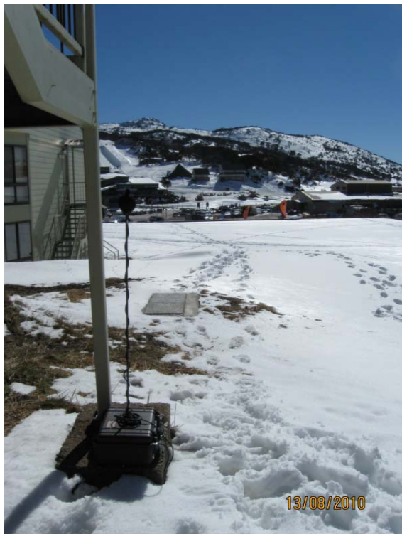
Figure 3 Noise logger in position.
