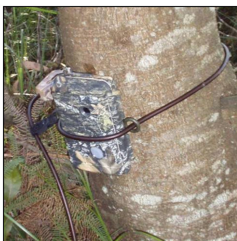
Figure A5-2: Camera unit with passive infrared trigger, secured to a tree with a non-slip cable
