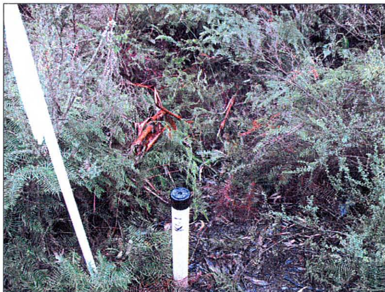
Photograph 1 – Piezometer type to be installed.
