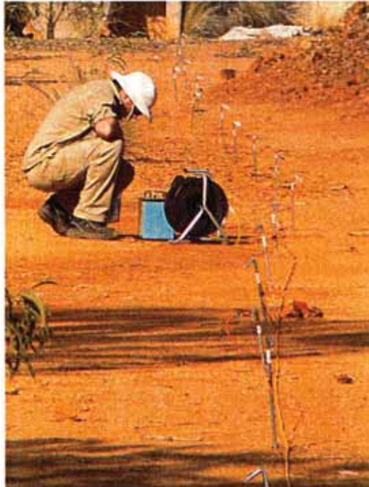
Figure 1. Resistivity Profiling (Source: AlphaGeoscience, 2009)
