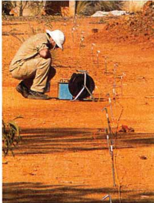
Figure 1. Resistivity Profiling (Source: AlphaGeoscience, 2009)
