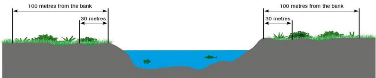
Figure 2: Measuring distance from the bank of an incised watercourse
