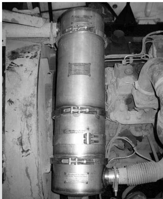
Exhaust treatment devices are being fitted to diesel vehicles to reduce particle emissions.
