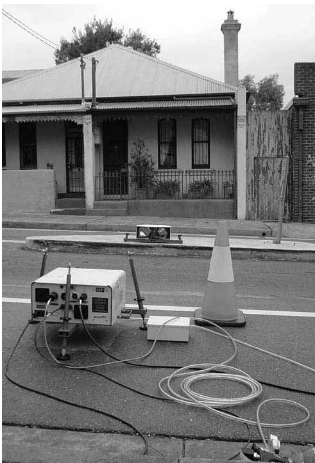
Smog Dog measures pollutants from vehicle exhaust pipes.
