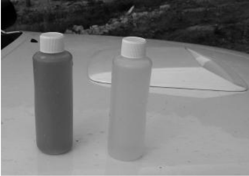
DECCW negotiated a pollution reduction program with Delta Electricity to reduce the turbidity of liquids being discharged into Cocks River. The bottle on the left shows samples before treatment, the bottle on the right shows samples after treatment.
