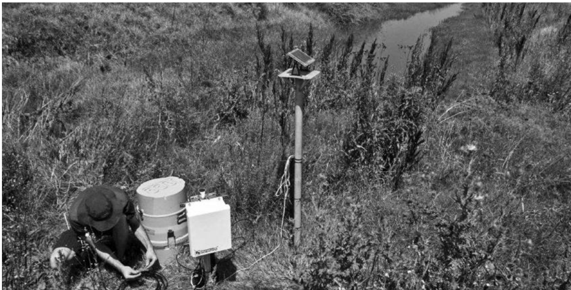
Automated water stations log runoff amounts and collect samples from farms as part of the Lower Hawkesbury–Nepean River Nutrient Management Strategy.
