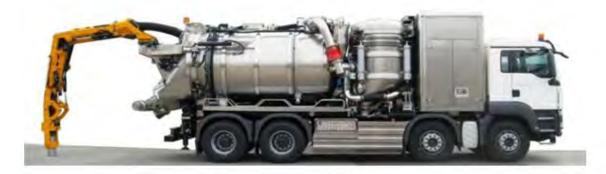
Tank / Debris - capacity 11 cubic metres
