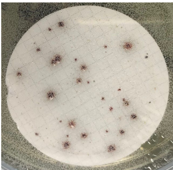
Figure 2 Enterococci colonies counted in the laboratory using membrane filtration technique for testing water samples
