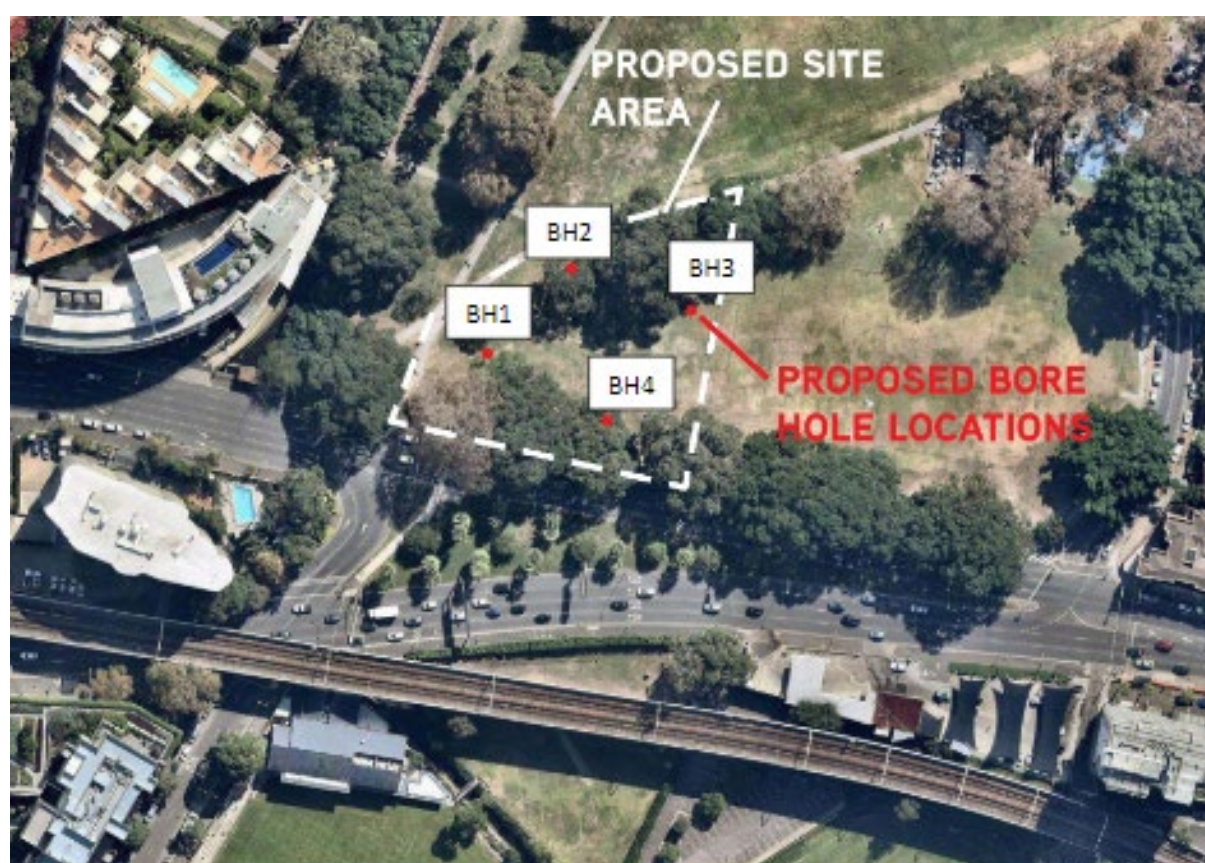
Figure 3.3 Aerial photograph with borehole locations, prepared by Fortify Geotech. (Source: Fortify Geotech 2019, Figure 2, p10)
