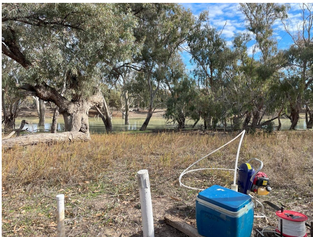
Figure 4: Typical groundwater sampling setup. Site 28 on the Great Darling Anabrach (Source: G Hose 2025)
