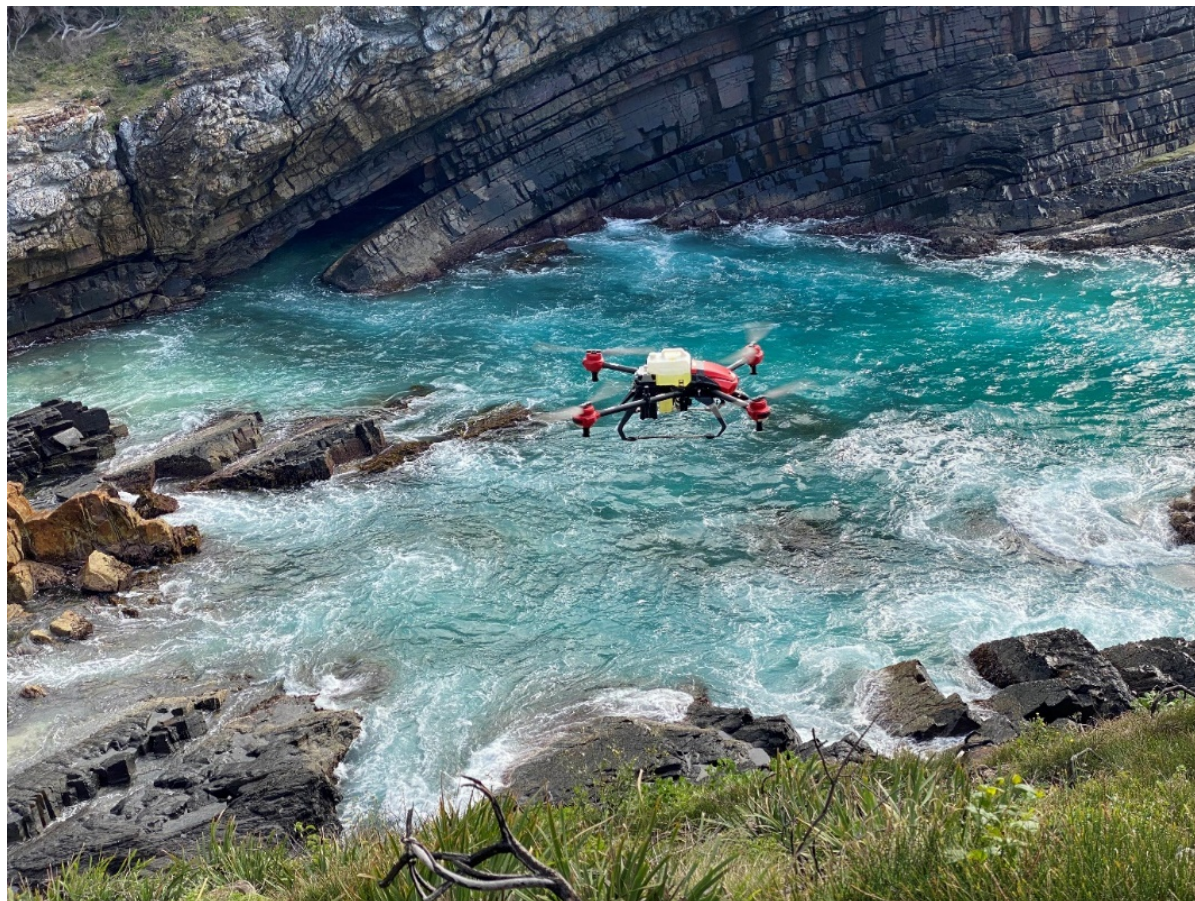
Figure 5 RPA spraying around inaccessible cliff line areas
