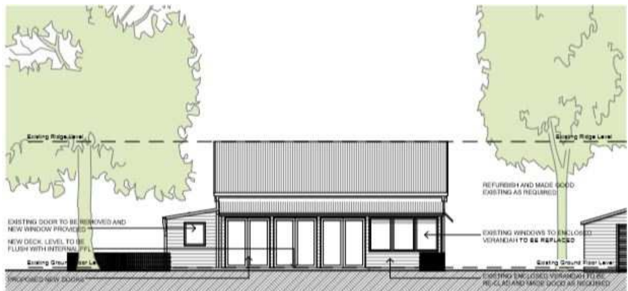
Figure 20 – 33 Green Point Cottage Proposed South Elevation
