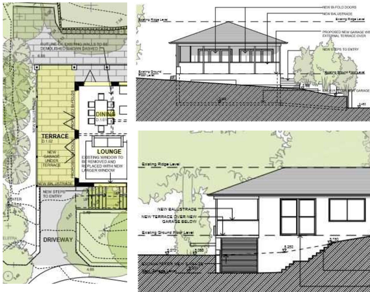
Figure 04 – 33 Cliff Road excavation Excavation limited to the driveway and garage areas
