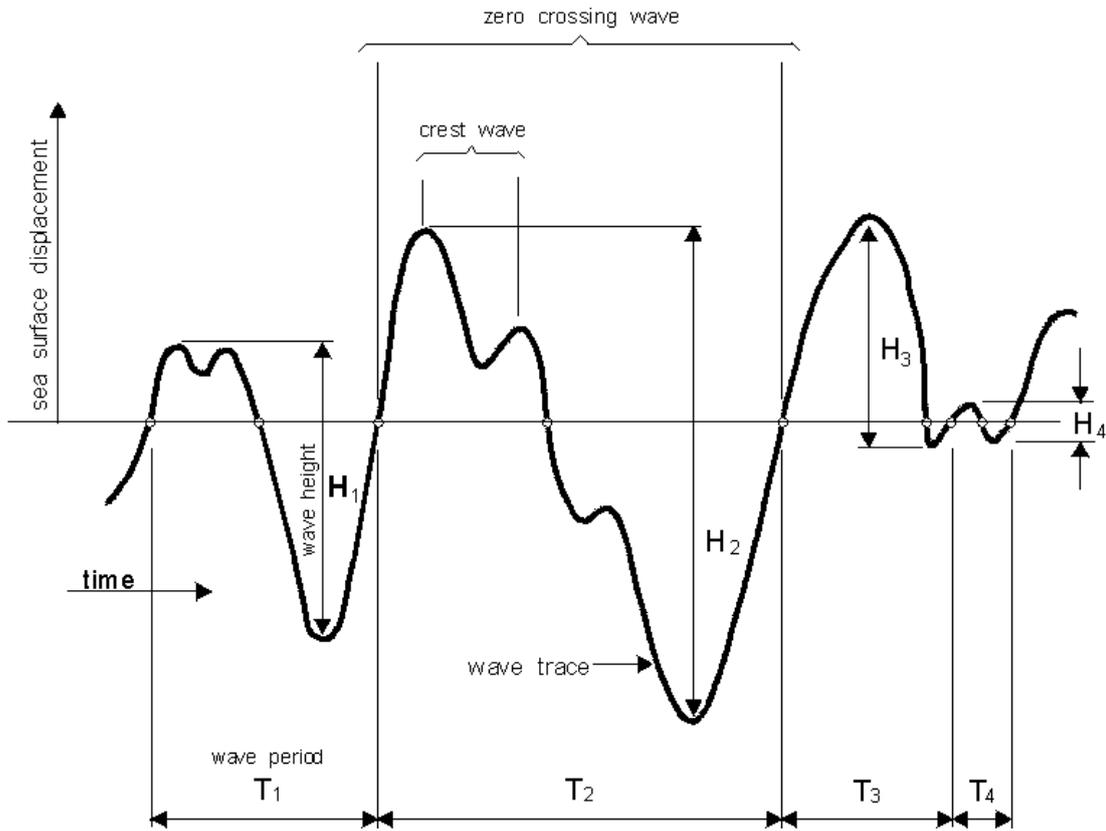
Example of wavy water surface and definitions of wave parameters
