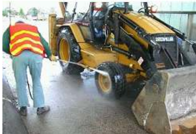
Figure 3. Wash down with high-pressure hose
