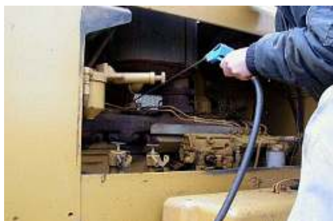
Figure 4. Clean down with compressed air
