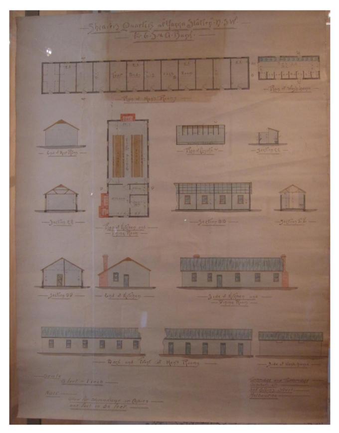
Figure 2.15 Architectural drawing prepared for the construction of the Shearers Quarters built in 1911. The architects were Tunbridge and Tunbridge of Melbourne. Source: Yanga Archives. On display in the Cook's Cottage exhibition.
