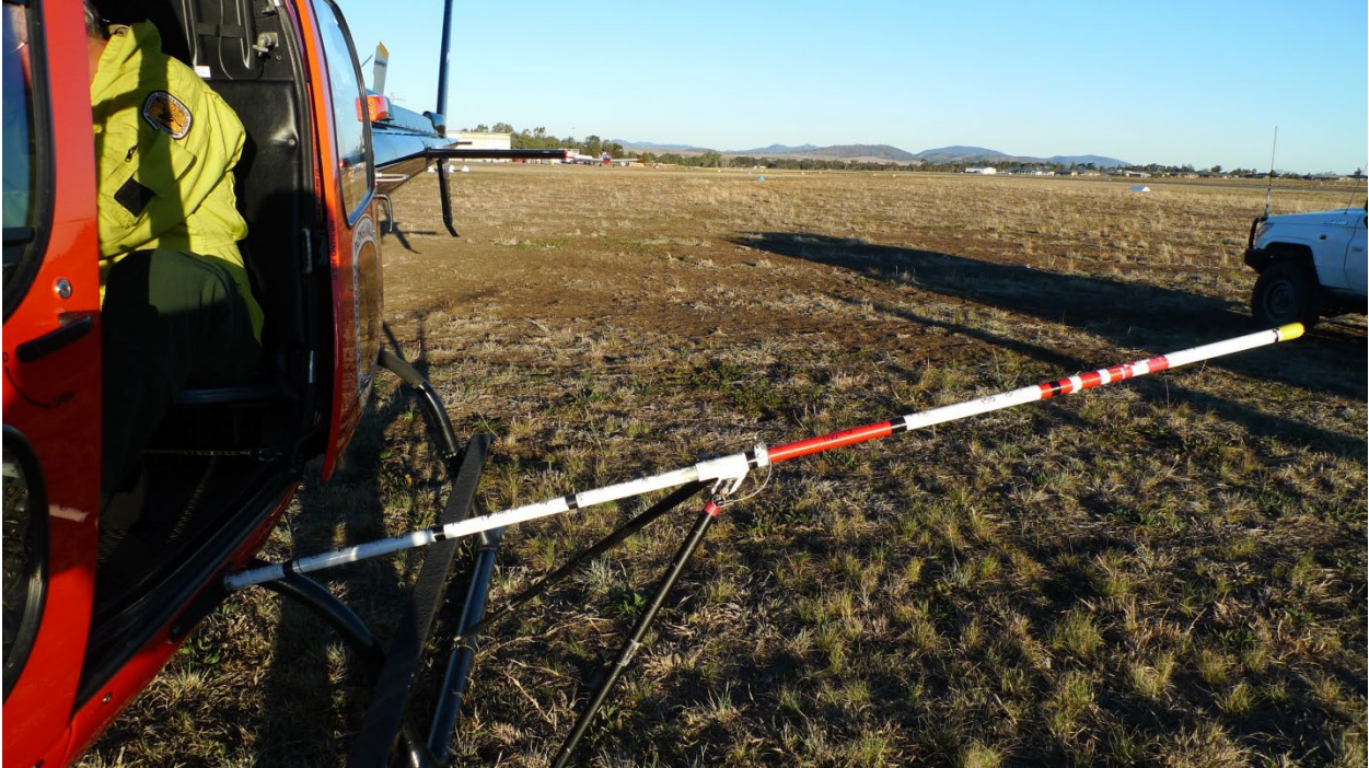
Fig. 6 Sighting boom mounted on the left-hand side of a Eurocopter AS350B3 Écureuil helicopter. The perpendicular distance classes used in the surveys (0-20 m, 20-40 m, 40-70 m, 70-100 m and 100-150 m) are indicated by the black bands on the boom.
