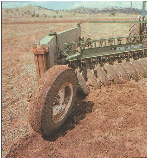
Overcultivation with implements, such as the disc plough, is a major cause of soil structure decline.
