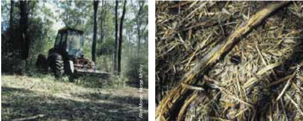
Surface mulching using a tritter [left] keys mulch into the surface to aid stability and revegetation [right]
