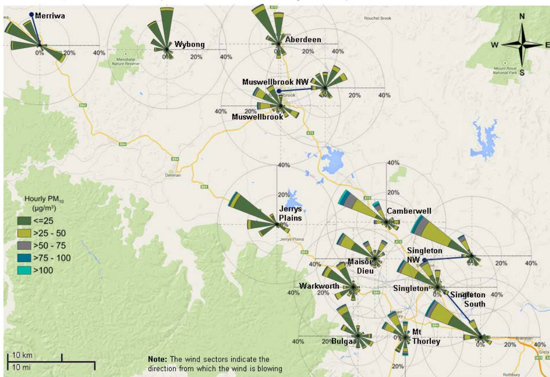
Figure 3 Hourly PM 10 pollution rose map for the Upper Hunter region for winter 2018
